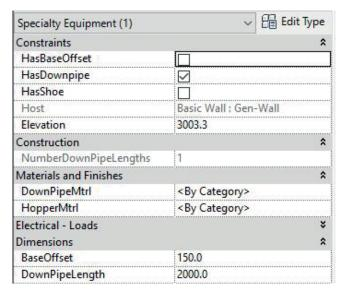
'HasBaseOffset': This feature will enter a predertmined figure to calculate the base offset. Once selected the 'BaseOffset' parameter in the 'Dimenions' category will control the overall offset distance from the downpipe.
